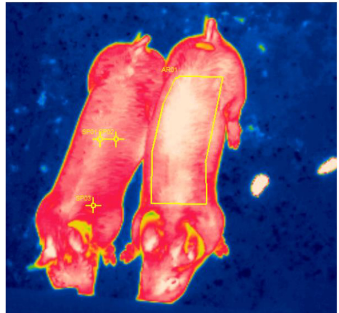
Fig. 2. Screenshot of a thermal image from the software FLIR ThermoCAM Researcher 2.10 Pro. The rectangular area on the back of the pig marks the region of interest (ROI). On the rear of the right pig, at the base of the tail, the silver spray mark for identification can be seen. Copyright: SRUC.
